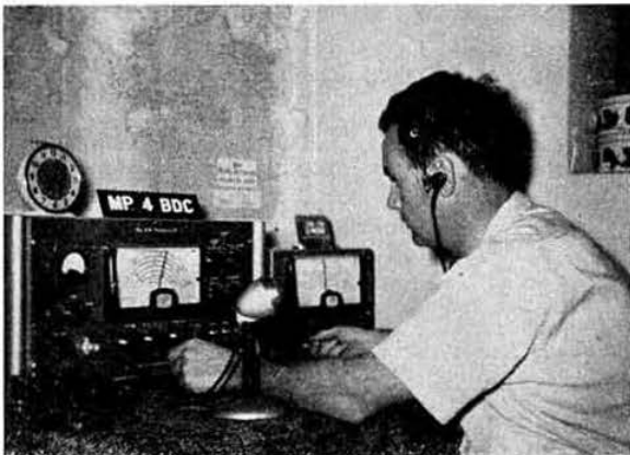
Frank Peacock operating MP4BDC in Bahrain. The equipment includes a K.W. Electronics Vanguard transmitter, a Geloso converter feeding into an R107 receiver, a two-band cubical quad for 21 and 28 Mc/s and a 7 Mc/s dipole. So far 102 countries have been worked. MP4BDC is usually on 21 Mc/s from 11.00-18.00 G.M.T. looking for G contacts.
